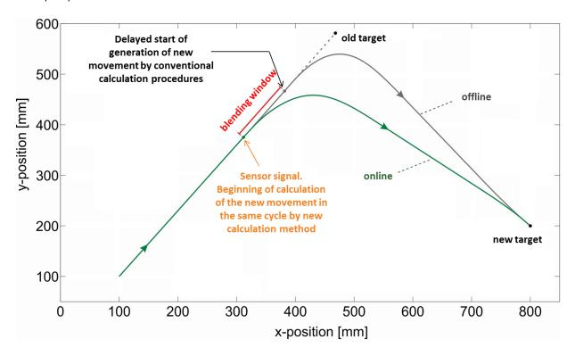
Both axis start to reach the old target position until an event in causing a change of the target position. A blending window is necessary in case of standard approach according to PLC Open Part 4 (grey line). KPA Motion calculates the multi-axis motion trajectories and starts the new movement starting in the cycle of the event (green line).
